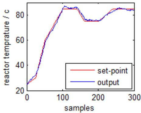
Fig.4 GMC reactor temperature (MAE=1.13at Std=0.15)
