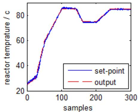
Fig.1 OE-MPC reactor temperature (10 batches)
