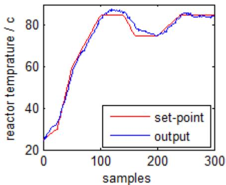
Fig.5 GMC reactor temperature (MAE=1.61 at Std=0.2)
