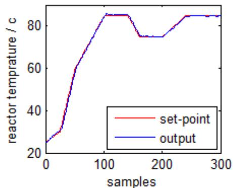
Fig.3 GMC reactor temperature (MAE= 0.48 at Std=0.01)
