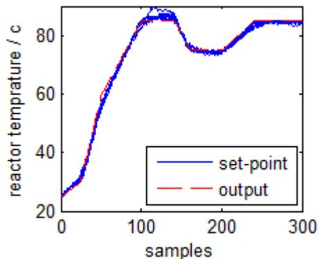
Fig.2 ARX-MPC reactor temperature (10 batches)
