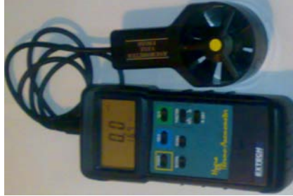
Figure (5): The Anemometer For measuring air speed, m/s.
