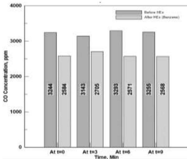
17. Carbon monoxide concentration before and after attaching the heat exchanger at 2700 rpm, FR=50% benzene.
