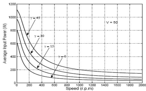
**Fig. 15** Variation of motor input power with speed at different values of advancing switching ON angle
