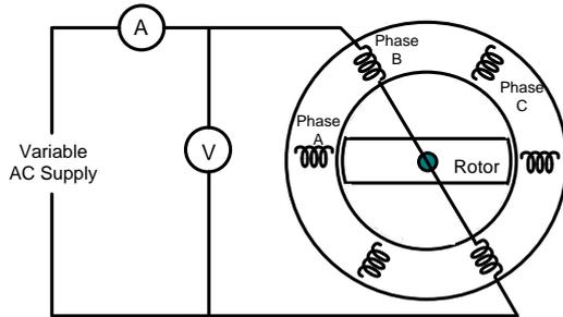
Fig. 2 Connection Diagram for inductance measurements
