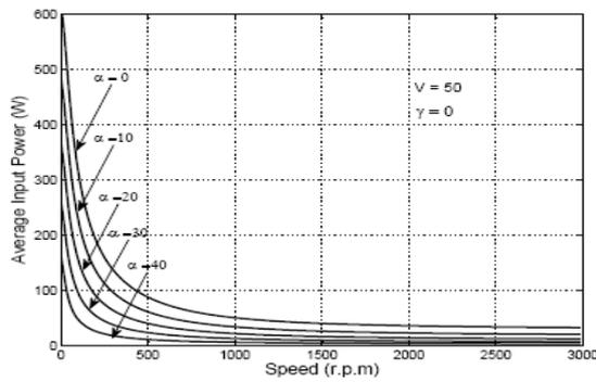
Fig. 21 Variation of input power with speed at different values of early switching OFF angle
