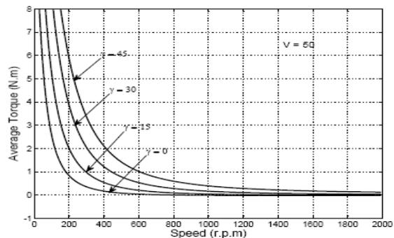
**Fig. 13** Variation of motor torque current with speed at different values of advancing switching ON angle
