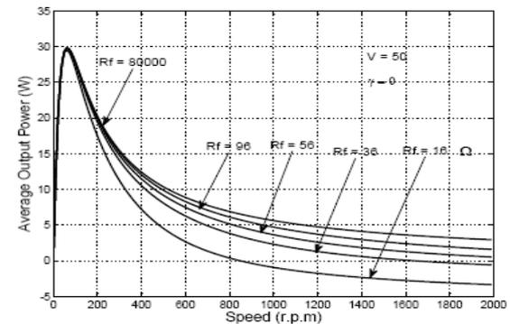
Fig. 25 Variation of output power with speed at different values of  $R_f$
