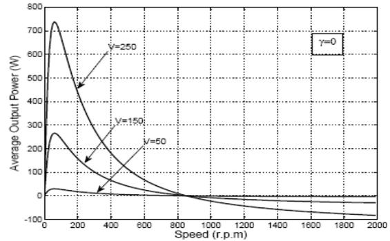
Fig. 8 Variation of output power with speed at different values of supply voltages
