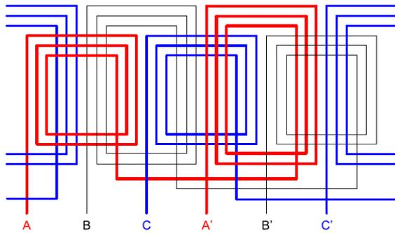
Fig. 1 Stator windings drawing
