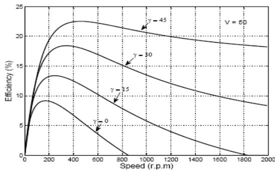
**Fig. 16** Variation of motor efficiency with speed at different values of advancing switching ON angle
