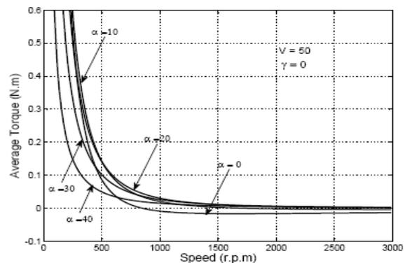
**Fig. 19** Variation of motor torque with speed at different values of early switching OFF angle
