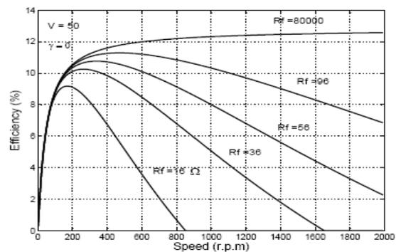
Fig. 26 Variation of motor efficiency with speed at different values of  $R_f$
