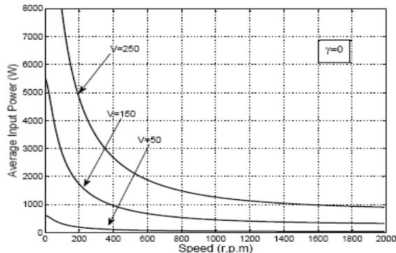
Fig. 9 Variation of input power with speed at different values of supply voltages
