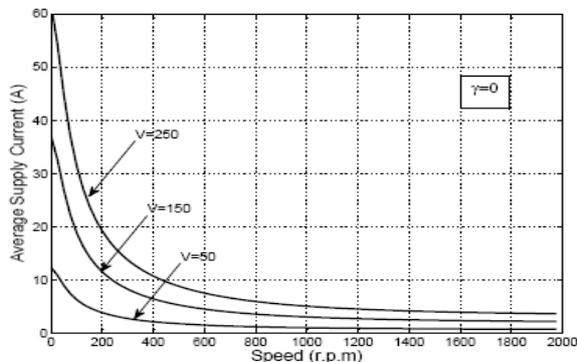
Fig. 5 Variation of supply current with speed at different values of supply voltages
