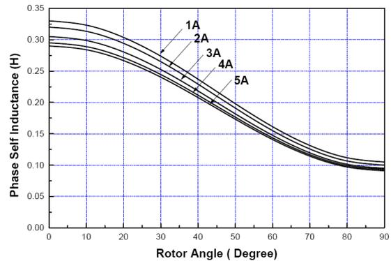
Fig. 3 Variation of phase self inductance with rotor angle at different currents
