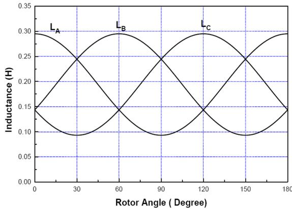
Fig. 4 Variation of phases inductances with rotor position
