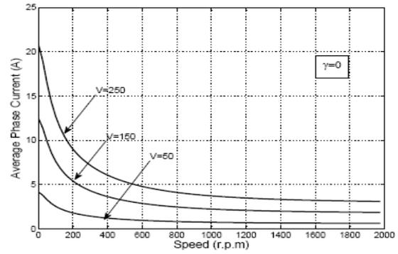
Fig. 6 Variation of motor phase current with speed at different values of supply voltages
