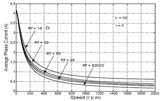
Fig. 23 Variation of phase current with speed at different values of  $R_f$
