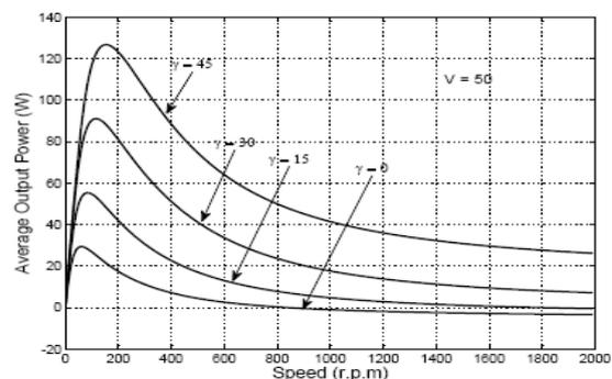
**Fig. 14** Variation of motor output power with speed at different values of advancing switching ON angle
