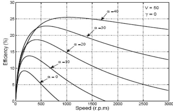
Fig. 22 Variation of motor efficiency with speed at different values of early switching OFF angle
