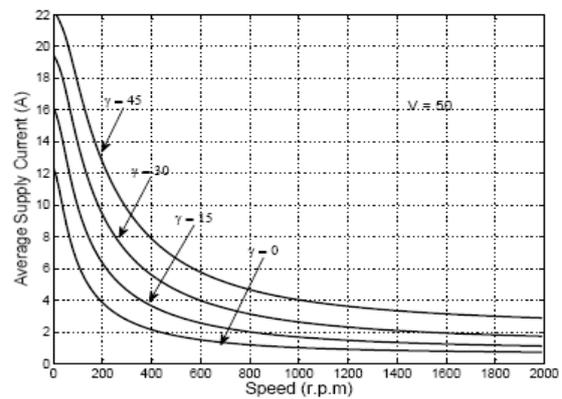
**Fig. 11** Variation of supply current with speed at different values of advancing switching ON angle
