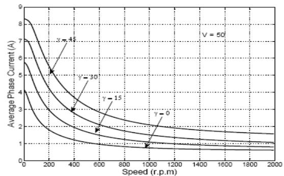
**Fig. 12** Variation of motor phase current with speed at different values of advancing switching ON angle
