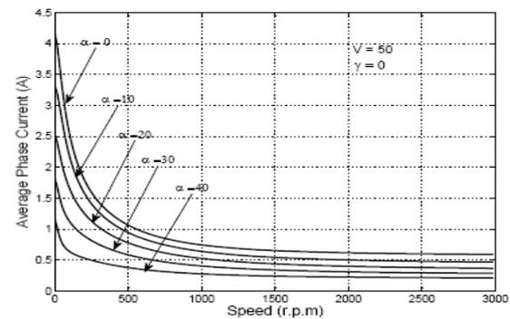
**Fig. 18** Variation of motor phase current with speed at different values of early switching OFF angle
