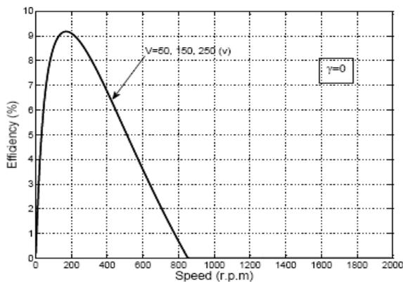
**Fig. 10** Variation of motor efficiency with speed at different values of supply voltages
