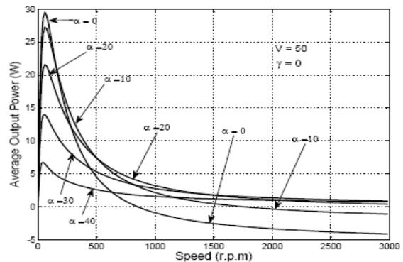
**Fig. 20** Variation of output power with speed at different values of early switching OFF angle
