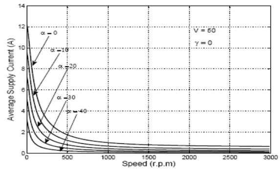
**Fig. 17** Variation of supply current with speed at different values of early switching OFF angle
