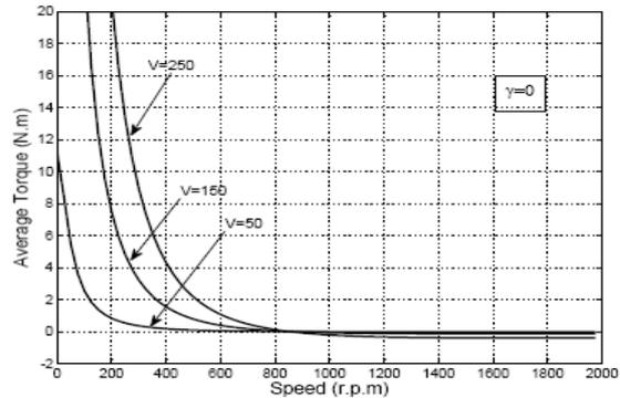
Fig. 7 Variation of total torque with speed at different values of supply voltages
