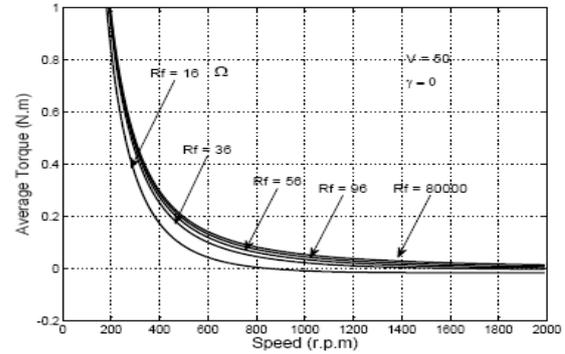
Fig. 24 Variation of total torque with speed at different values of  $R_f$
