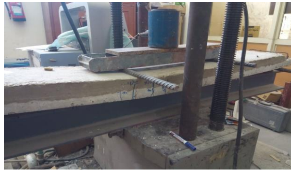
Fig. 2 Slab specimens test setup
