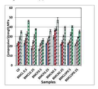
Figure (3): Compressive Strength for All Bacterial and Control Concrete mixes.
