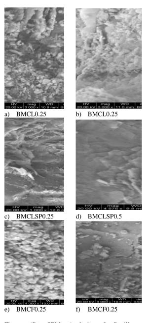
Figure (5): SEM Analysis of *Bacillus Megaterium* Bacterial Concrete (a), (b) 0.25% with Lactate Nutrition, (c), (d) Lactate Nutrition Using Super plasticizer, and (e), (f) 0.25% with Formate nutrition.
