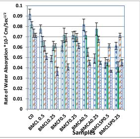
Figure (1): Rate of Water Absorption for Bacterial and Control Concrete after 24 hours.
