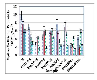
Figure (2): Capillary Permeability Coefficient (K) for Bacterial and Control Concrete after 24hours.
