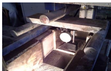
Figure (1) Flexure Test of Reinforced Laminates
