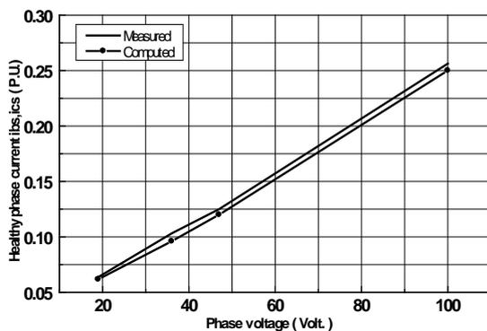
Fig.10 Measured and computed healthy phase currents against phase voltage at 25% fault ratio.
