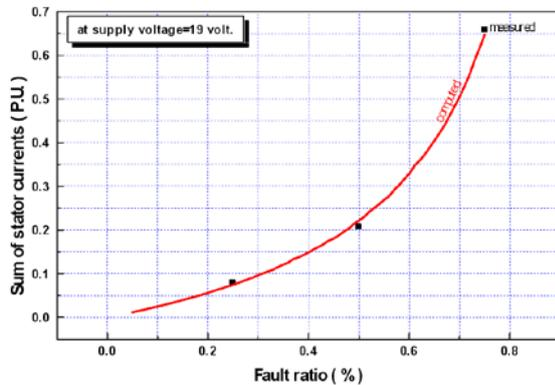
Fig.22 Sum of stator currents against fault ratio at supply voltage=19 volt.
