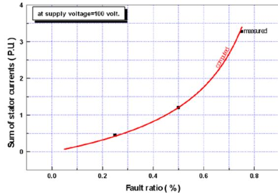
Fig.25 Sum of stator currents against fault ratio at supply voltage=100 volt.
