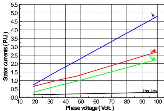
Fig.3 Stator currents against voltage at 50% fault ratio in phase A
