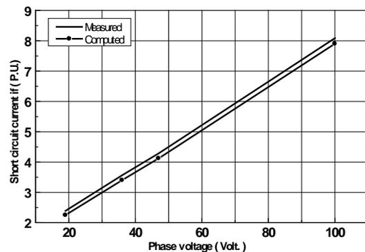
Fig.20 Measured and computed short circuit current against phase voltage at 75% fault ratio.
