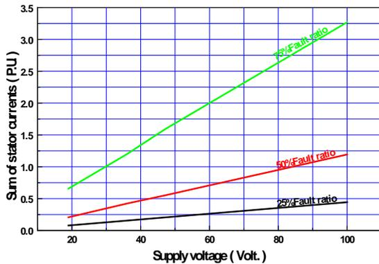
Fig.21 Sum of stator currents against supply voltage at 25%, 50%, 75% fault ratio
