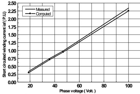
Fig.15 Measured and computed short circuited winding current against phase voltage at 50% fault ratio.
