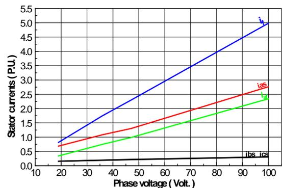
Fig.7 Stator currents against voltage at 50% fault ratio in phase A
