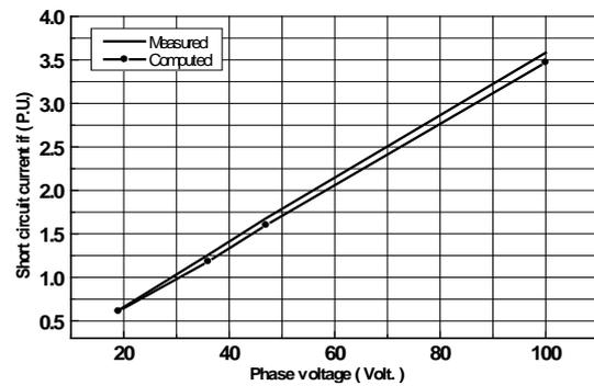
Fig.12 Measured and computed short circuit current against phase voltage at 25% fault ratio.
