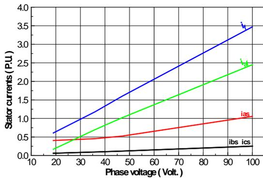
Fig.2 Stator currents against voltage at 25% fault ratio in phase A
