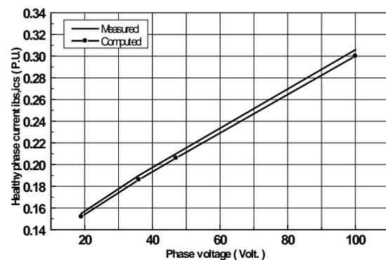
Fig.14 Measured and computed healthy phase currents against phase voltage at 50% fault ratio.
