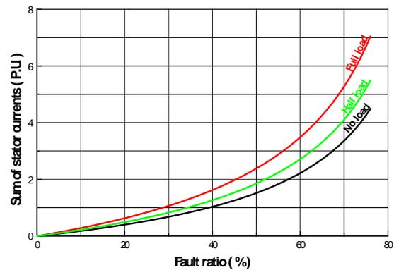
Fig.26 Sum of stator currents at different values of load torque at rated voltage.
