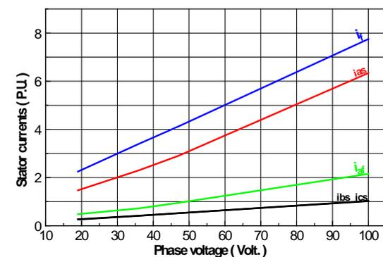
Fig.4 Stator currents against voltage at 75% fault ratio in phase A
