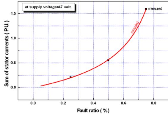
Fig.24 Sum of stator currents against fault ratio at supply voltage=47 volt.
