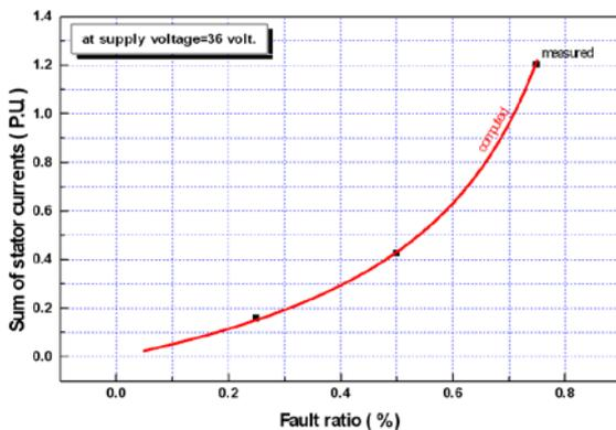
Fig.23 Sum of stator currents against fault ratio at supply voltage=36 volt.
