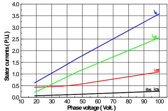
Fig.6 Stator currents against voltage at 25% fault ratio in phase A
