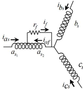
**Fig.1** Stator circuit of induction motor with inter-turn fault in the phase a.
