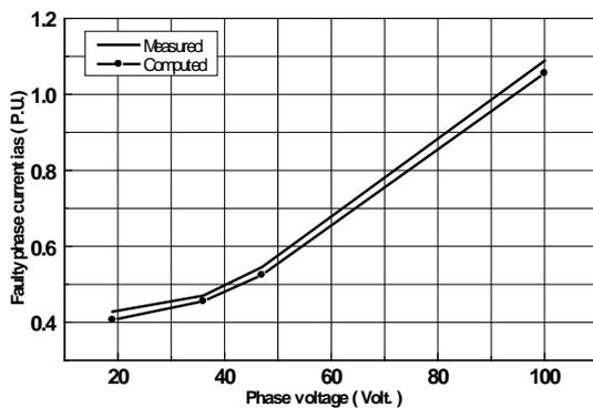
Fig.9 Measured and computed faulty phase current against phase voltage at 25% fault ratio.
