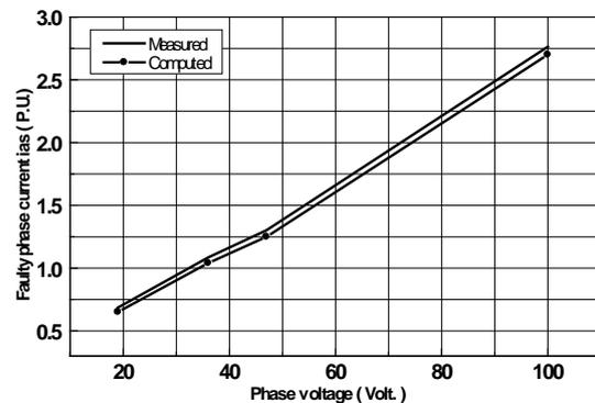
Fig.13 Measured and computed faulty phase current against phase voltage at 50% fault ratio.
