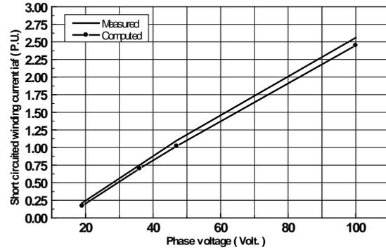
Fig.11 Measured and computed short circuited winding current against phase voltage at 25% fault ratio.
