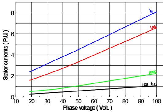
Fig.8 Stator currents against voltage at 75% fault ratio in phase A.
