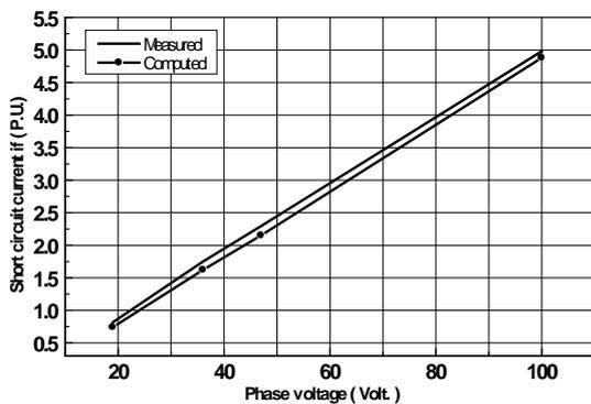
Fig.16 Measured and computed short circuit current against phase voltage at 50% fault ratio.
