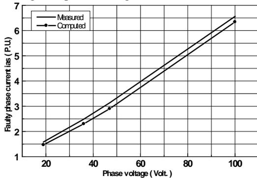
Fig.17 Measured and computed faulty phase current against phase voltage at 75% fault ratio.
