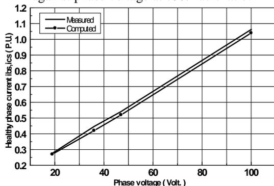
Fig.18 Measured and computed healthy phase currents against phase voltage at 75% fault ratio.
