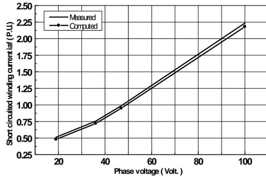
Fig.19 Measured and computed short circuited winding current against phase voltage at 75% fault ratio.
