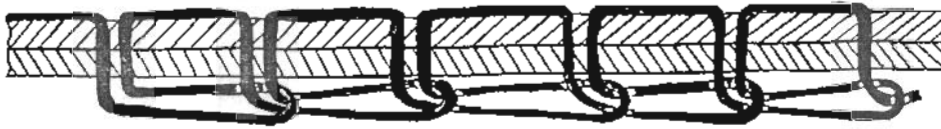
Fig. 1(b): Single-thread chain stitch seam.
