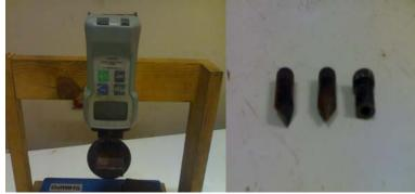
Figure (5): Digital hardness and shear force gauge.
