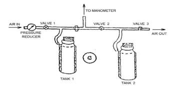
Figure (3): laboratory apparatus used for measuring jojoba seeds porosity.
