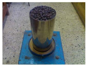
Figure (2): Bulk density meter with shaker.
