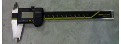
Figure (1): Digital vernier caliber
