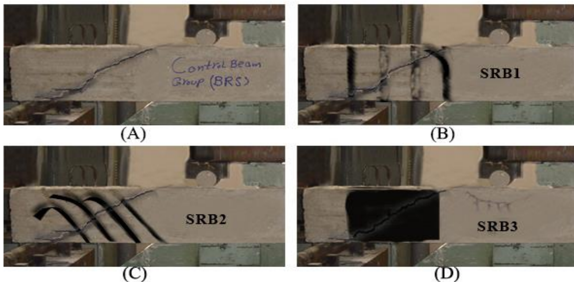
Figure 11: De-bonding and shear failures in group SRB.
