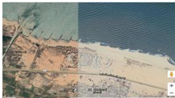
Figure 2- Protection works along the coast of Baltim resort (detached breakwaters and groins) west of Kitchener drain
