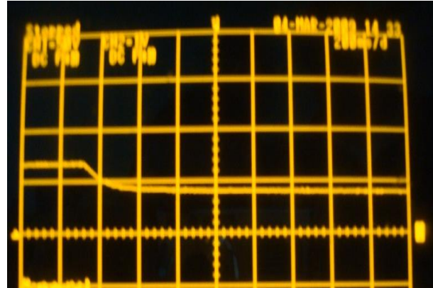
Figure (11-b) Variations of motor input voltage due to change in Load torque from (0.06: 0.036) .N.m.
