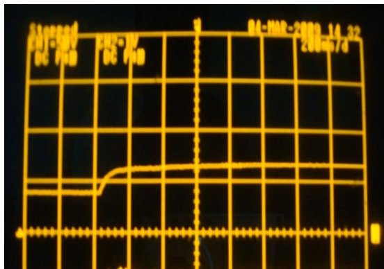
Figure (10-a) Variations of the motor input voltage due to change in Load torque from (0.036: 0.06) .N.m
