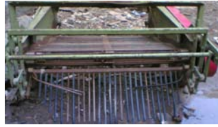
Fig (3): The vibrator and elevator before development
