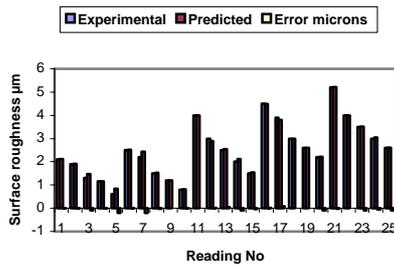
Fig. 5 Validation of GA model for surface roughness
