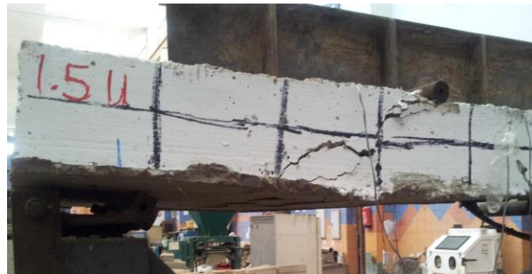
Fig. (6) Failure mode of slab S1-1.5U
