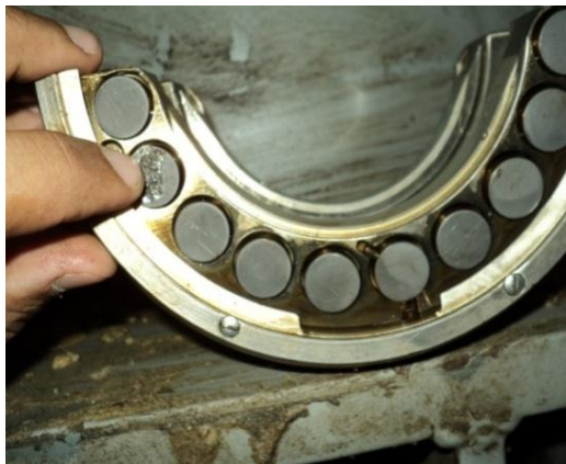
Fig.11. Defects at the thrust bearing pads
