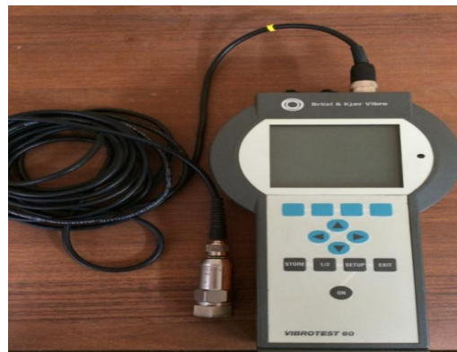
Fig. 3 Vibration data collector (B&amp;K VIBRO 60)
