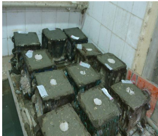
Fig (4) Hollow core in concrete cubes after casting
