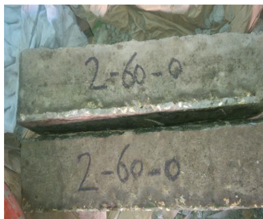
Fig (6) Concrete beams after casting and coding
