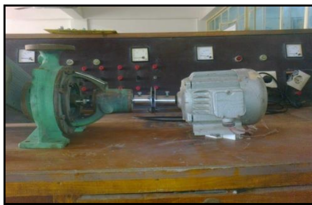
Figure (3) : The photo of the pump connected with (DC) motor.
