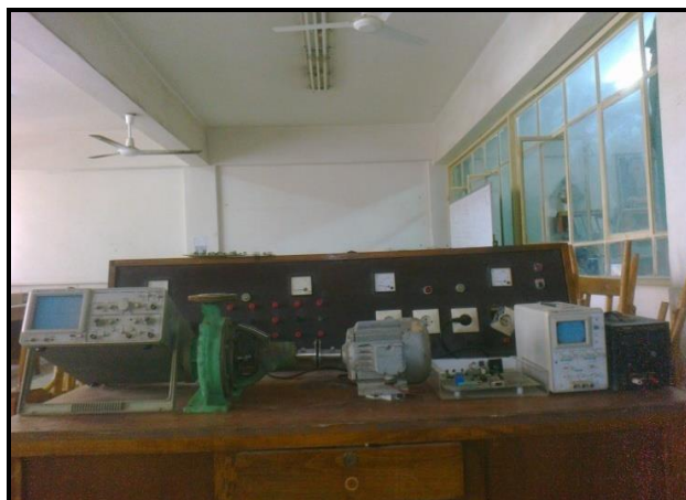
Figure (4) : Experimental arrangement for measurement of MPPT device and pump connected with DC Motor
