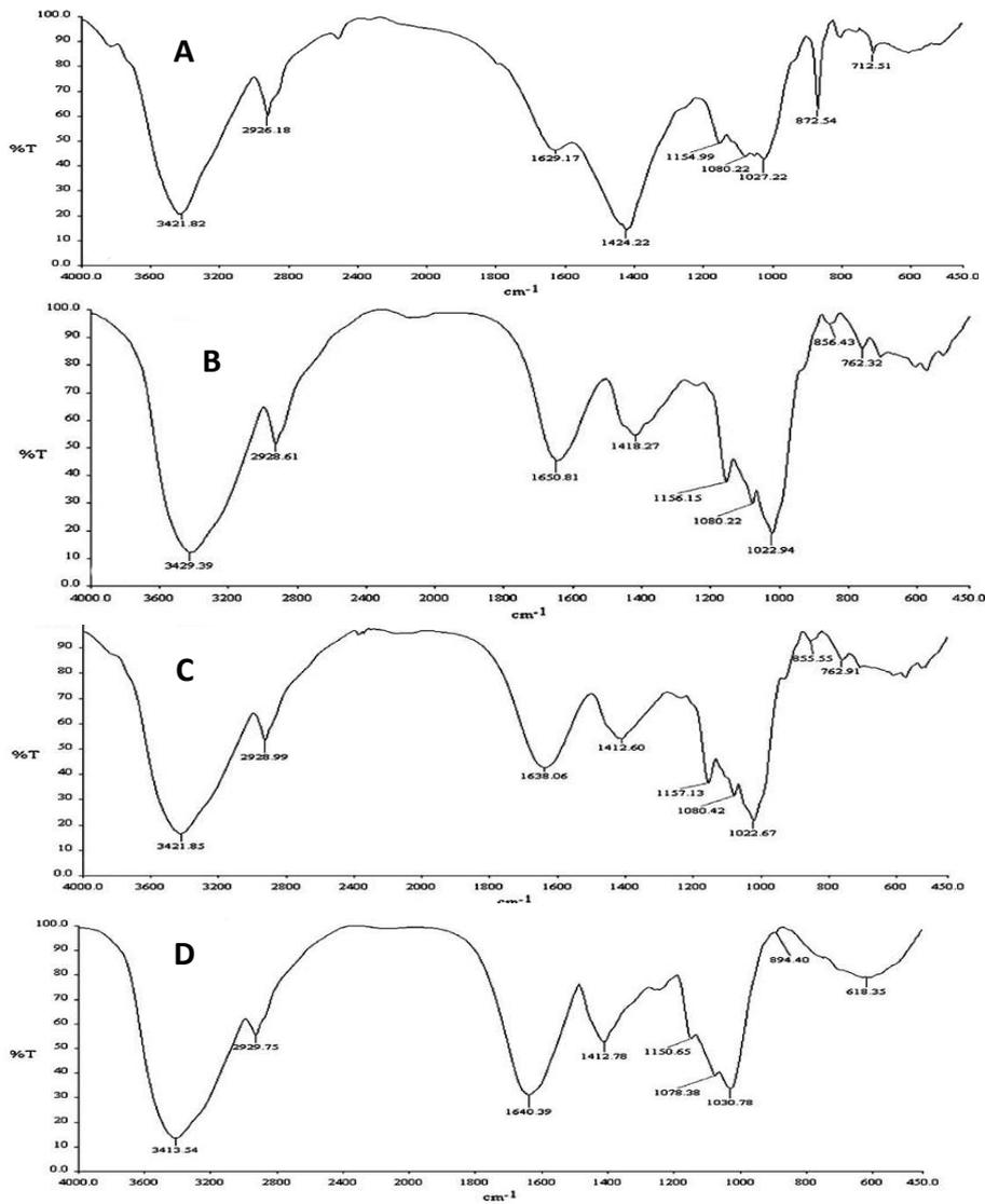
**Fig.3 FTIR spectra of the polysaccharide fractions (GP1(A), GP2(B),GP3(C) and GP4(D))**
