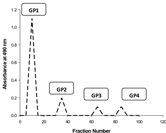
**Fig.1 Ion exchange column chromatogram of eluted crude polysaccharide (CP) on DEAE-cellulose (300 x25 mm).**
