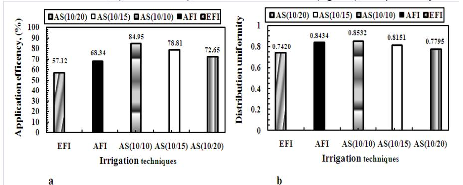
**Fig. (3): Water application efficiency and distribution uniformity under different irrigation techniques.**
