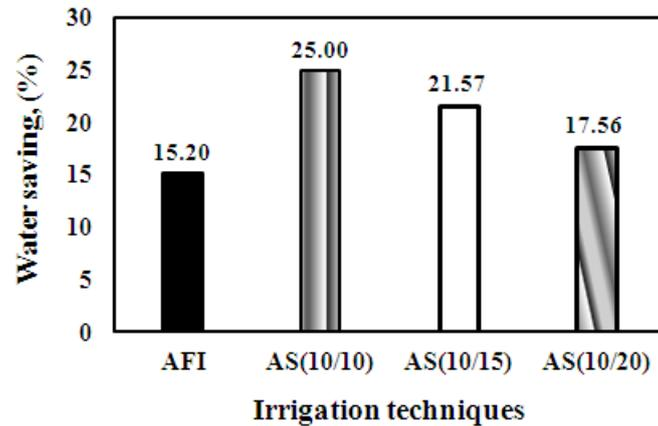
**Fig. (2): Water saving under different irrigation techniques relative to EFI treatment.**
