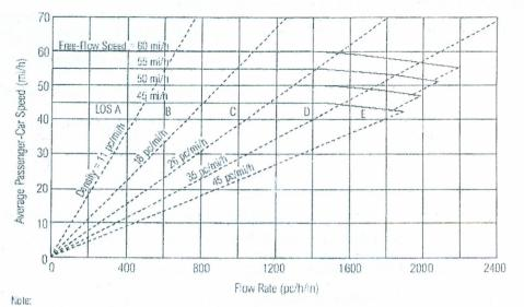
Maximum densities for LOS E occur at a v/c ratio of 1.0. They are 40, 41, 43, and 45 pc/mi/In at FFS of 60, 55, 50, and 45 mi/h, respectively. Capacity varies by FFS. Capacity is 2,200, 2,100, 2,000, and 1,900 pc/h/ln at FFS of 60, 56, 50, and 45 mi/h, respectively.
