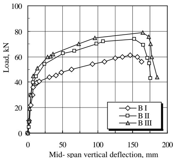
Fig. 2 Load-deflection curves RC beams tested at RT
