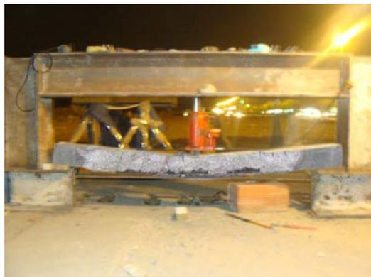
**Photo 1** Normal HPSCC beam, BI, after exposing to fire
