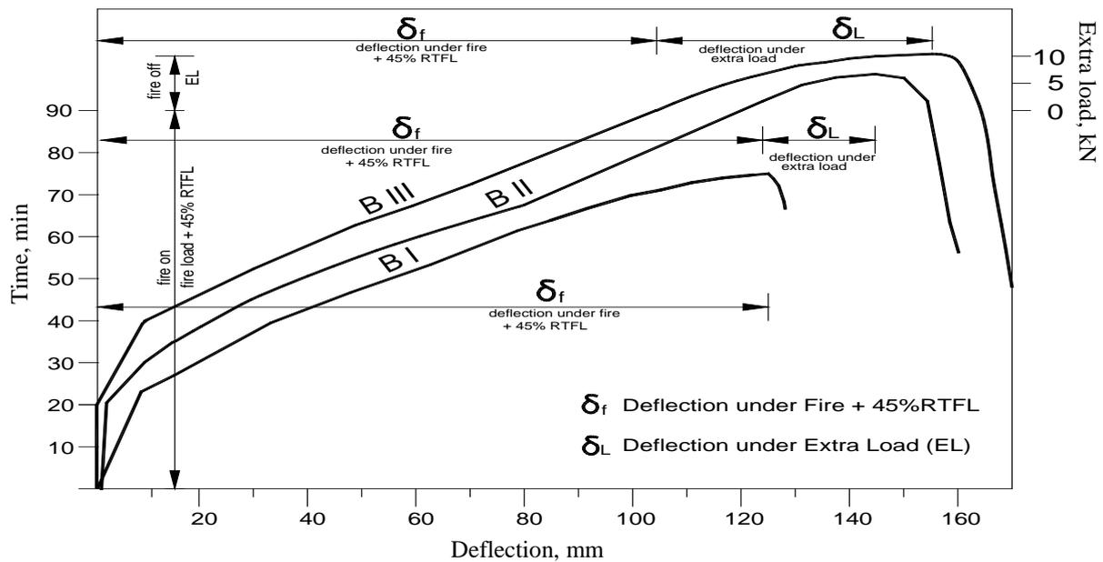
Fig. 4 Time-deflection curves for different RC beams
