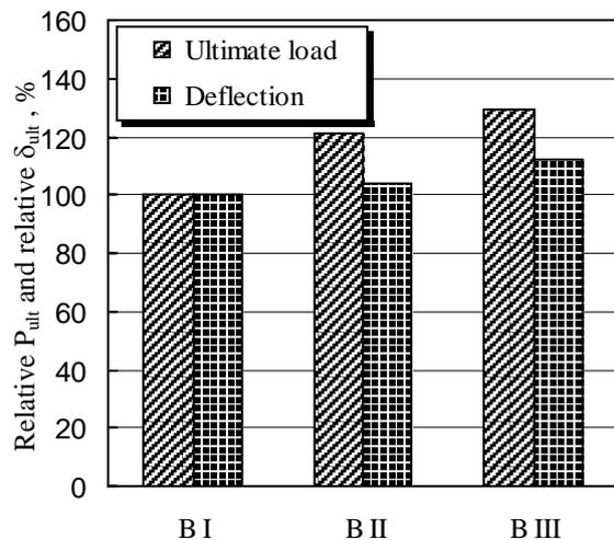
Fig. 3 Relative ultimate loads and corresponding relative deflection for RC beams at RT
