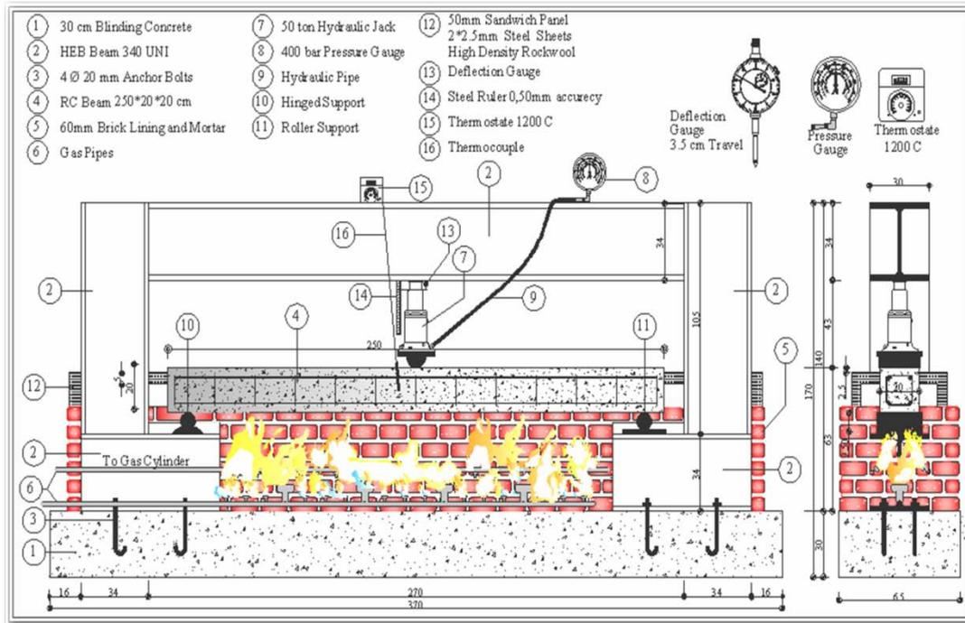
Fig. 1 Test setup for RC beams under gas furnace
