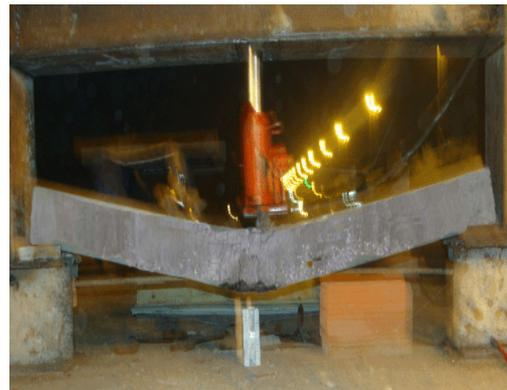
**Photo 2** HPSCC beam, BIII, after exposing to fire
