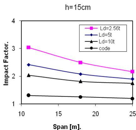
Fig.8: The relation between span length, load and IF for h=15cm.
