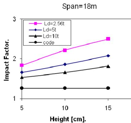
Fig.9: The relation between obstacle height and IF for 18m span.
