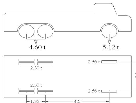
Fig.5: Vehicle configuration.
