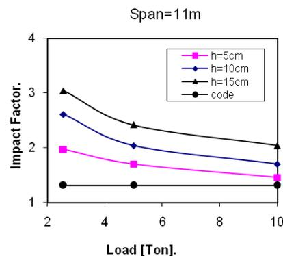
Fig.7: The relation between vehicle load and the IF for 11m span.
