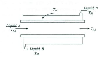
counter-currently around the tube. The temperature of liquid B decreases from  $T_{B1}$  to  $T_{B2}$ .
