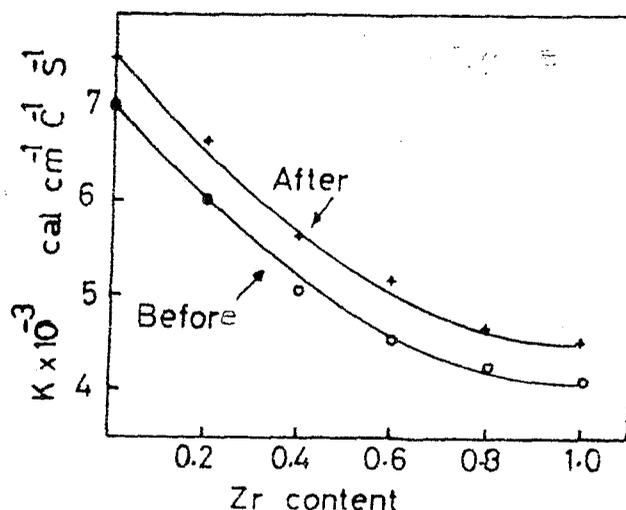
Fig. 5. Thermal conductivity vs Zirconium content, measured at temperature 50°C.
