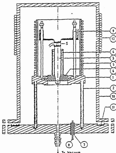
Fig. 1. Cross-section of the apparatus used for the thermal measurements.
