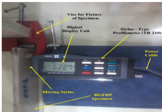
Figure 10- A Photograph of the Surface Roughness Measurement Setup of Drilled RGFRP Specimen
