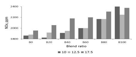
Fig. 9. NOx emission from diesel engine with different blended fuels
