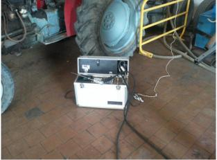
Fig. 4: The exhaust gas analyzer
