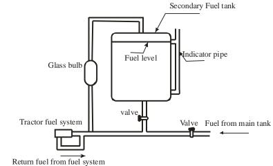
Fig. 3. schematic diagram for local manufactured fuel consumption meter
