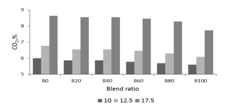
Fig. 7. CO<sub>2</sub> emission from diesel engine with different blended fuels
