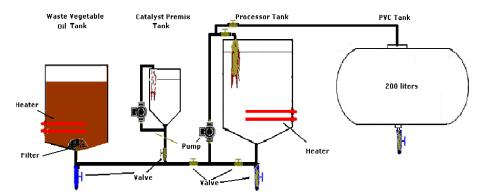
Fig. 1. Pilot biodiesel plant
