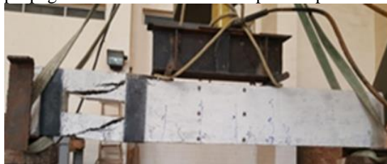
Fig. 8a Crack pattern for BSOST1
