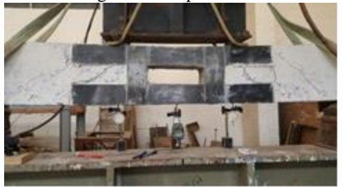
Fig. 9f Crack pattern for BMOC3
