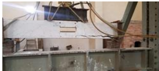
Fig. 9a Crack pattern for BMOST1
