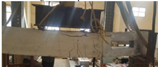
Fig. 8b Crack pattern for BSOST2
