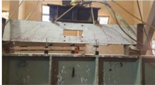
Fig. 9d Crack pattern for BMOC1
