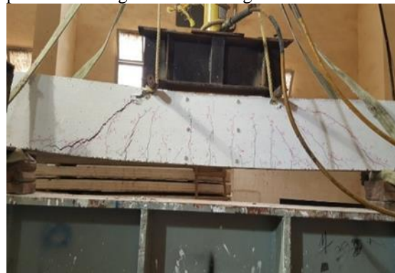
Fig. 7a Crack pattern for CB
