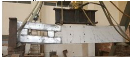
Fig. 8c Crack pattern for BSOST3
