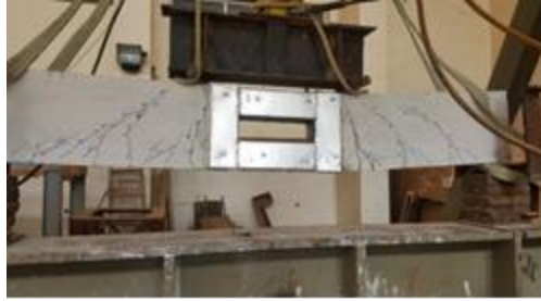
Fig. 9c Crack pattern for BMOST3
